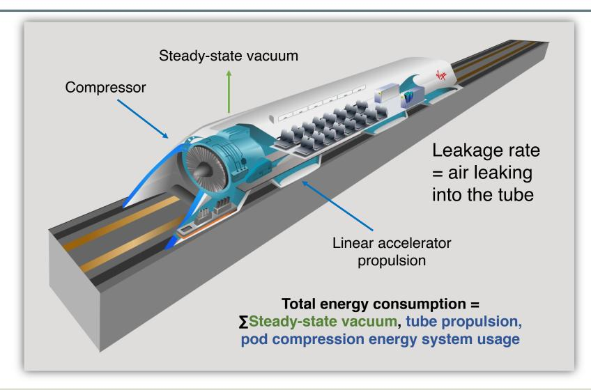
For a fixed leakage rate, there is an optimal operating pressure for the tube
