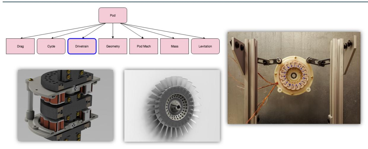
**Levitation:** computes the magnet mass and drag from the passive MagLev subsystem using 1<sup>st</sup> principal physics models
