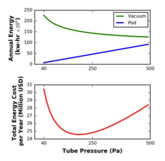
Leakage rate = 3 kg/s Optimal tube pressure = 190 Pa
