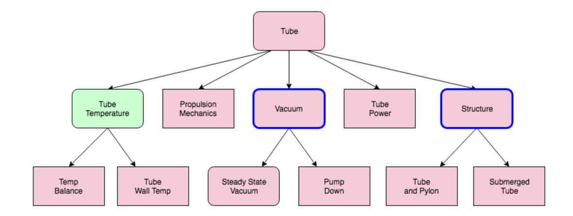
**Vacuum:** computes the energy usage for the pump-down and steady-state vacuum pump systems using 1D thermodynamics models
