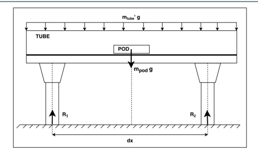
Underwater analysis is a tube, under a distributed buoyant load with point loads holding it down
